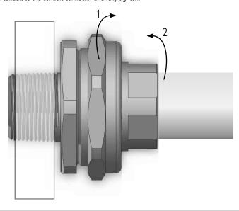
3. Fully tighten the nut (3) to ensure that the elements forming the serrated flamepath (2) are closely engaged.
